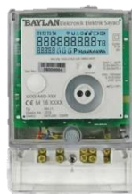
Figure 5. Electronic Energy Meter
